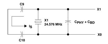
Figure 3–19. Load Capacitance for the PCI7x20 PHY
