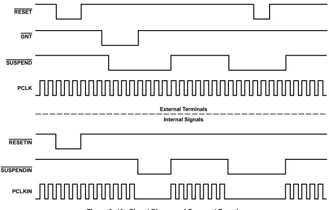
Figure 3–13. Signal Diagram of Suspend Function
