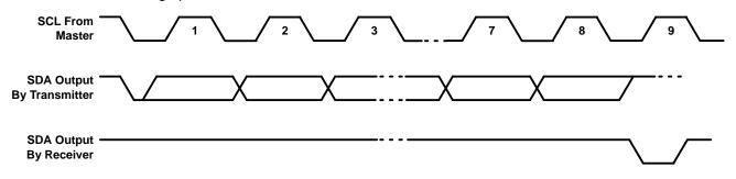
Figure 3–7. Serial-Bus Protocol Acknowledge
