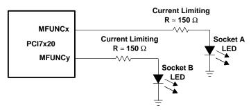
Figure 3–5. Two Sample LED Circuits
