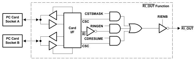
Figure 3–14. RI\_OUT Functional Diagram
