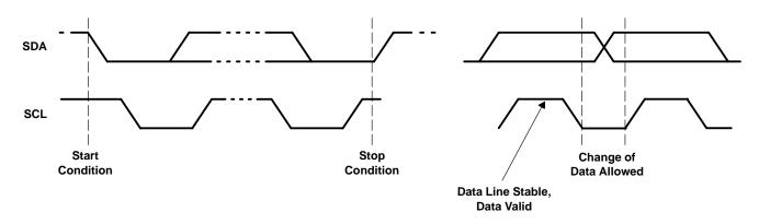
Figure 3–6. Serial-Bus Start/Stop Conditions and Bit Transfers
