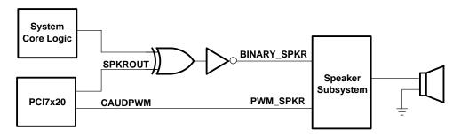
Figure 3–4. SPKROUT Connection to Speaker Driver
