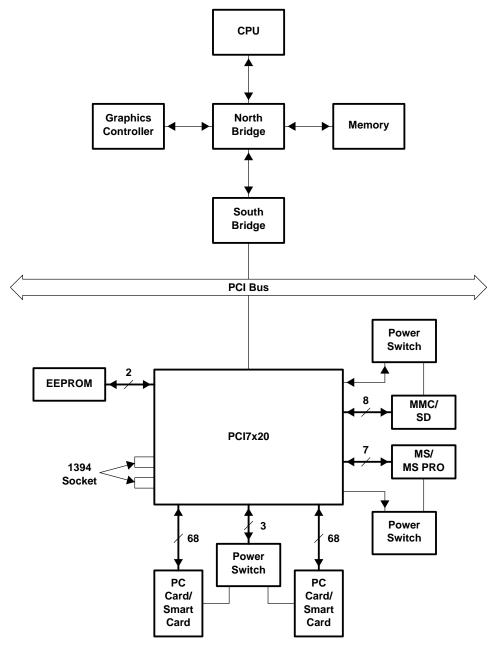
Figure 3–1. PCI7x20 System Block Diagram
